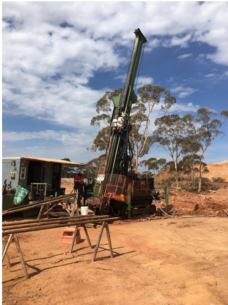
Figure 1: Diamond drilling Eureka open pit mine.
